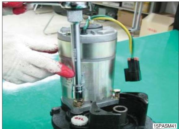
(6) Disassemble motor from actuator assy.
