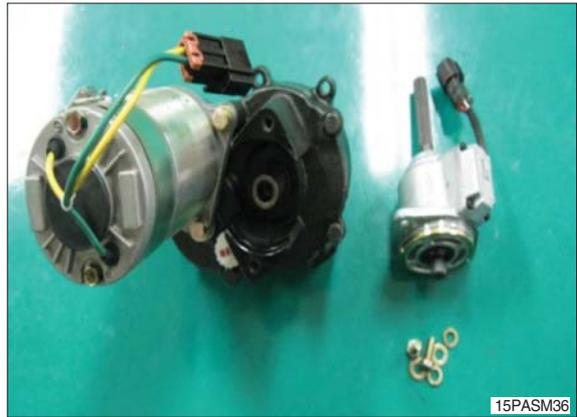
(4) Disassemble joint coupling which is assembled on torque sensor.
