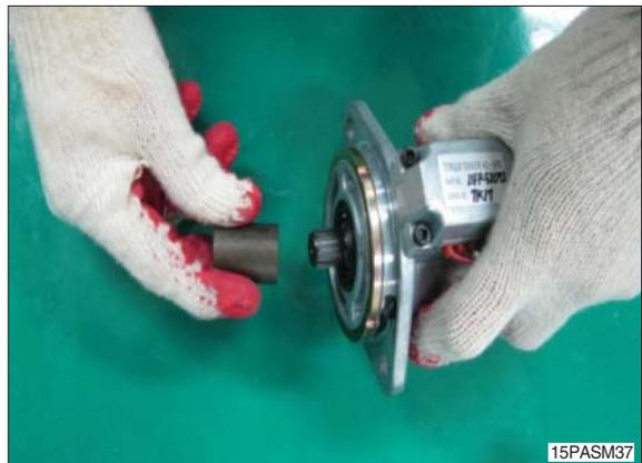
(5) Disassemble hexagon bolt (M8×25) which is assembled on motor by using the below tool.
